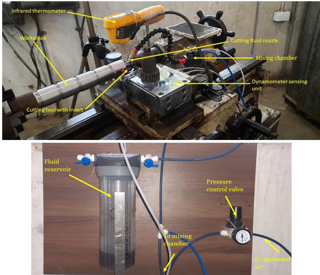
Figure 3.2 Experimental setup along with MQL system
